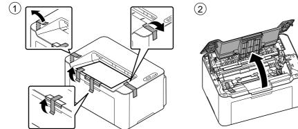
4. Remove the tape and packing ③. Grab the Drum Unit D ④ as shown and lift it from the Printer. (5) Place it on a sheet of paper on a flat surface.
