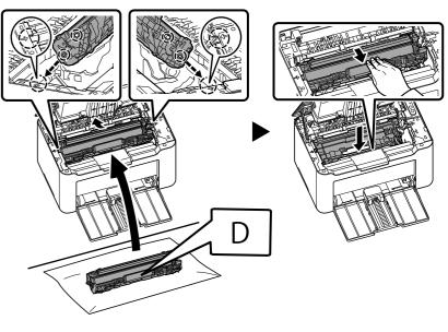
5. Open the front Paper Feeder 6 and remove the packing sheet that protects the drum  $\overline{O}$ .
